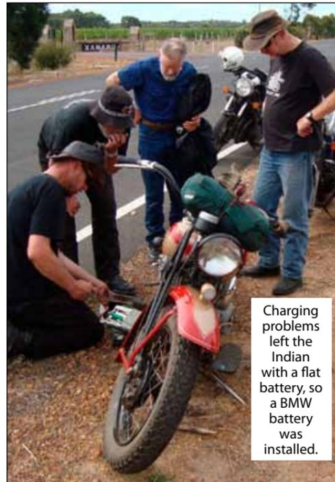
Charging problems left the Indian with a flat battery, so a BMW battery was installed.
